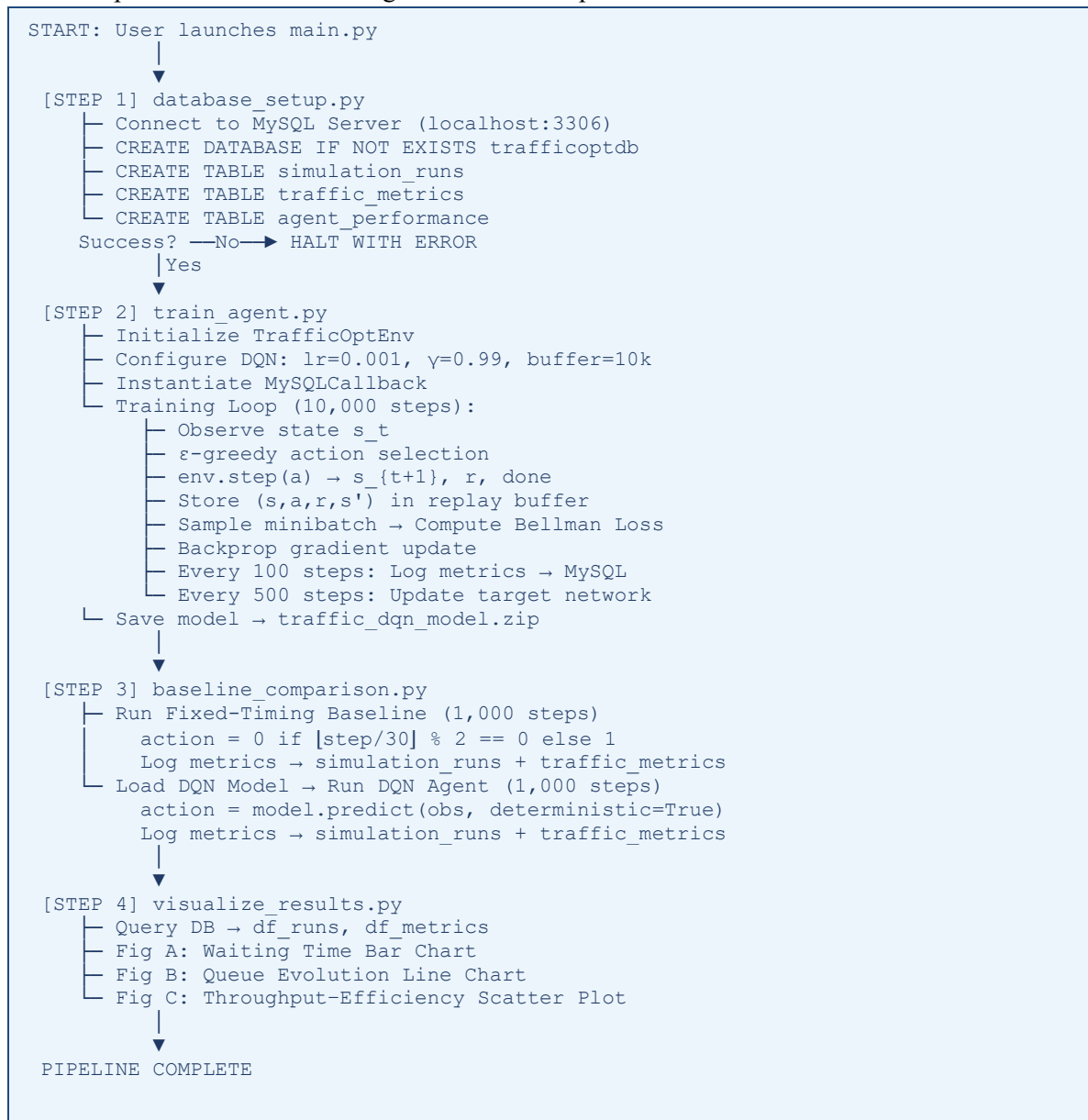
Figure 2: Workflow Diagram — Complete operational flow of the TrafficOpt RL pipeline from system initialization through training, evaluation, and visualization generation
